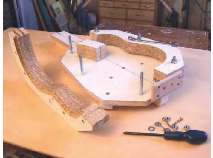
▲ Pic.8 The mould varnished on the inside and ready to use
